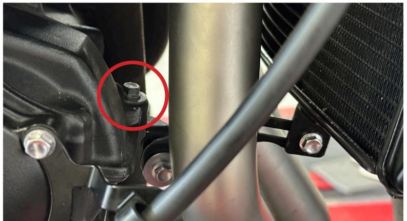
**If the header of cylinder 1 is at a distance of less than 6–8 mm from the horn bracket welded to the radiator, proceed as follows:**
